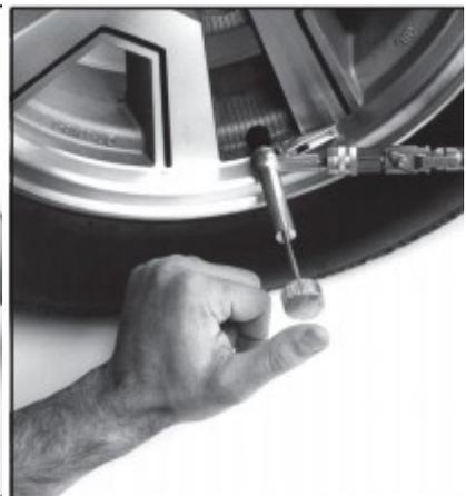
Put your thumb on top of the VCR's knob applying downward pressure. With the other hand, unscrew the knob (about 25 revolutions) or until the core clicks
