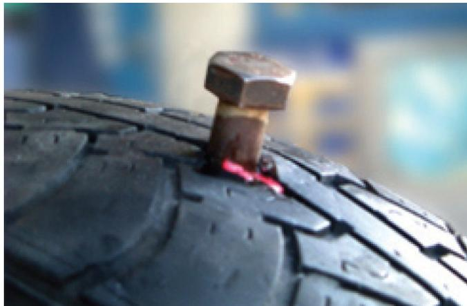
As the rubber recovers, the wound closes and the strength of the tyre holds the repair in place. The specialized polymers and fibres form a clot, producing an airtight repair. The small amount of Punctureseal that penetrates through the wound, past the belts and out through the tread area, is referred to as a repair or clot. Once exposed to the atmosphere, the repair/clot begins a systematic chemical cure (another proprietary attribute from the Punctureseal R&D Team).
