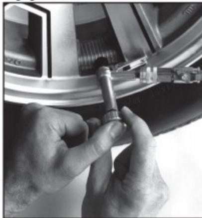
With the core stored up into the VCR chamber, Punctureseal can easily be installed without losing air pressure.
