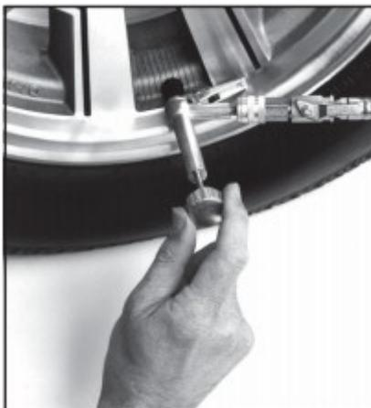
Squeeze the trigger and place the VCR onto to the valve stem. Position of the tyre is not critical
