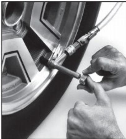
**Very Important** Push the plunger/knob down to engage the valve core. Slowly turn the knob, lining up on the valve core. Press down to engage and lock onto the core
