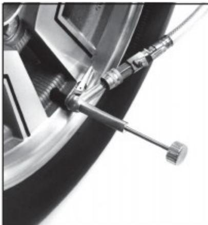
Release the pressure from your thumb, thereby allowing the tyre's air pressure to push the knob, shaft and valve core up into the chamber.
